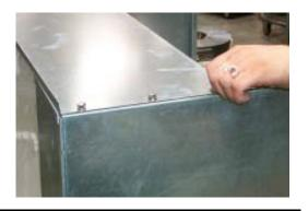
After assembling the Wash-It sink, seal all bolts and seams from the inside of the sink using the provided silicone sealant.
