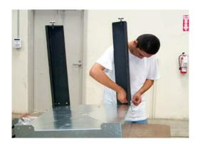
Loosely fasten the leg braces between the two back legs and two front legs with the smooth side facing out using four bolts, washers, and nuts.
