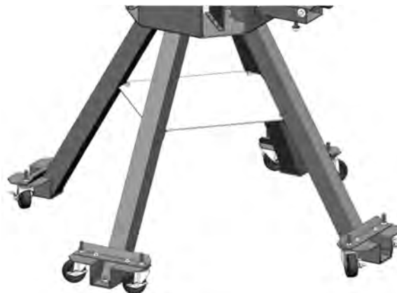
Drop Down Wheel Set Installed
