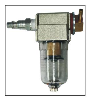
There is a screw fitting located on the bottom of the bowl to drain the filter. With the air on loosen this fitting but do not remove it. Air will force any fluid through the fitting. When all fluid has been evacuated tighten the fitting.
