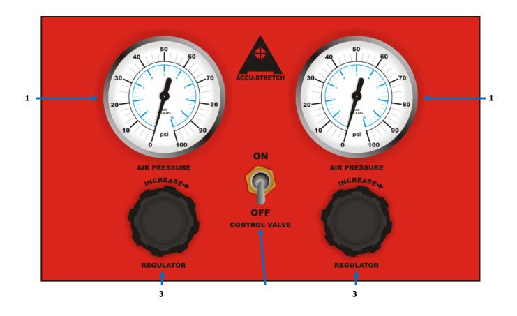
**1.** Gauges: These display air pressure being applied to stretch boxes. The one to the left reads pressure for stretch boxes #1 and #3. The one on the right reads pressure for stretch boxes #2 and #4. This reads in PSI, not newtons.
