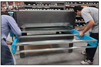
2. With another person and two flanged nuts in hand, lift up the infeed and insert it into the four exposed hex bolts.
