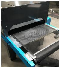
3. Run the belt under the infeed roller and then above the tension roller and above the lower support. Then feed the belt through the lower portion of the chamber and out the outfeed side of the dryer.
