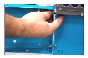
3. While holding the outfeed, hand tighten the nut to the top hex bolt first. Hand tighten a second nut to the bottom hex bolt. Be sure to do step three on both sides simultaneously.
