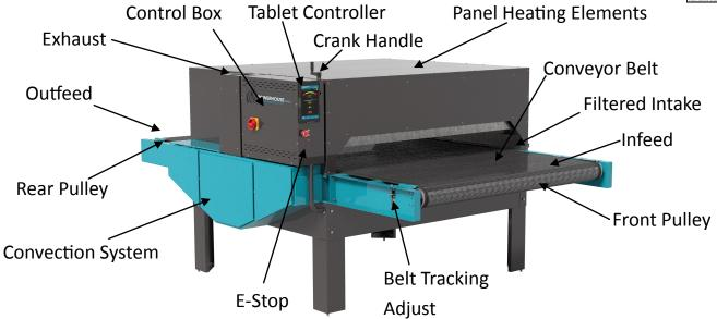
Panel Heating Elements Underneath the top panel there are three infrared radiant panel heating elements that are controlled by the tablet controller. They can cure plastisol, water-based ink, and any evaporative cured ink. They are capable of heating up and cooling down within seconds.
