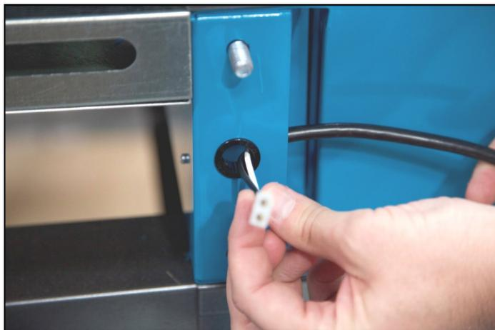
1. On the outfeed side, take the belt drive motor cable and feed it through the hole located at the edge of the arm.
