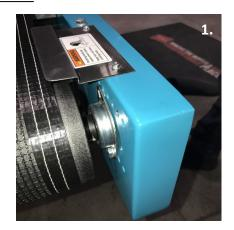
2. Feed the belt from the outfeed side of the dryer, through the top of the chamber. Pull the belt through the infeed side and over the infeed roller.
