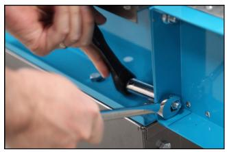
4. Using the 9/16" wrench on the top of the bolt and the 9/16" socket wrench on the nut, tighten all four hex bolts.
