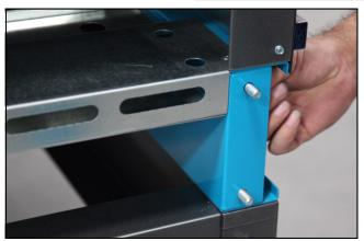
1. The infeed arm (the arm without the cooling table), must be attached to the side with the tablet. Insert a hex bolt and washer into the four holes where the arm will connect. Make sure the hex bolt is facing out and exposed.
