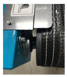
1. Once the belt is pinned together, you will need to reinstall the nuts and bolts for the infeed roller. Move the roller bearing back into place so that the bottom bolt and top bolt are aligned. The bolt will go into the bearing from the roller side of the arm and the nut will tighten down on the outside of the arm.
