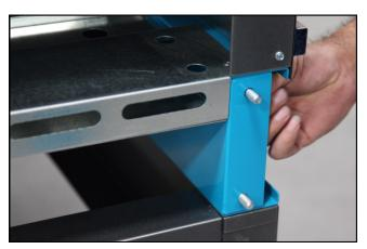
1. The outfeed arm (the arm with the cooling table), must be attached to the side opposite of the tablet. Insert a hex bolt and washer into the four holes where the arm will connect. Make sure the hex bolt is facing out and exposed.
