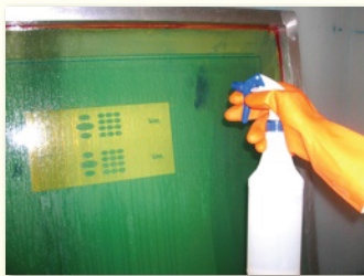
1. Spray ENVIROWASH® on both sides of screen.
