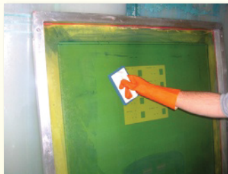
2. Scrub screen with non-abrasive pad or brush.
