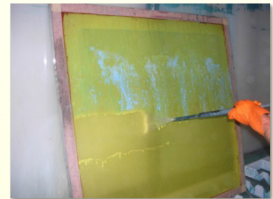
Step 3. High pressure rinse - starting at bottom.
