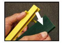
**REMOVE:** place the holder in your left hand, with your right hand peel the blade out of the holder's slot.
