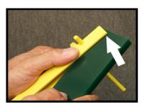
**INSTALL:** place the holder in your left hand, use your right hand to align one end of the blade to one end of the holder and push.
